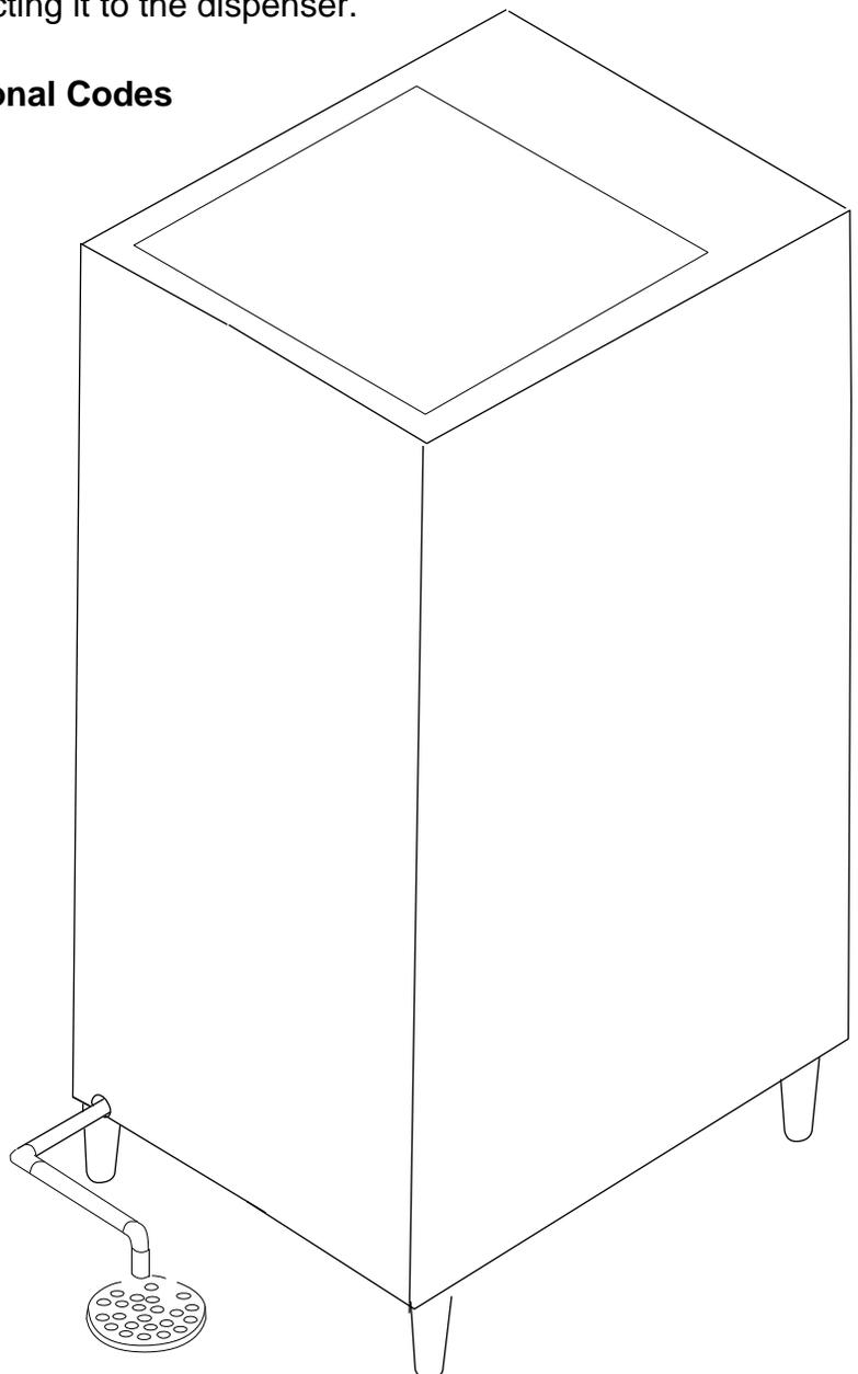
**Caution: Do not use a condensate pump in place of a floor drain.**
