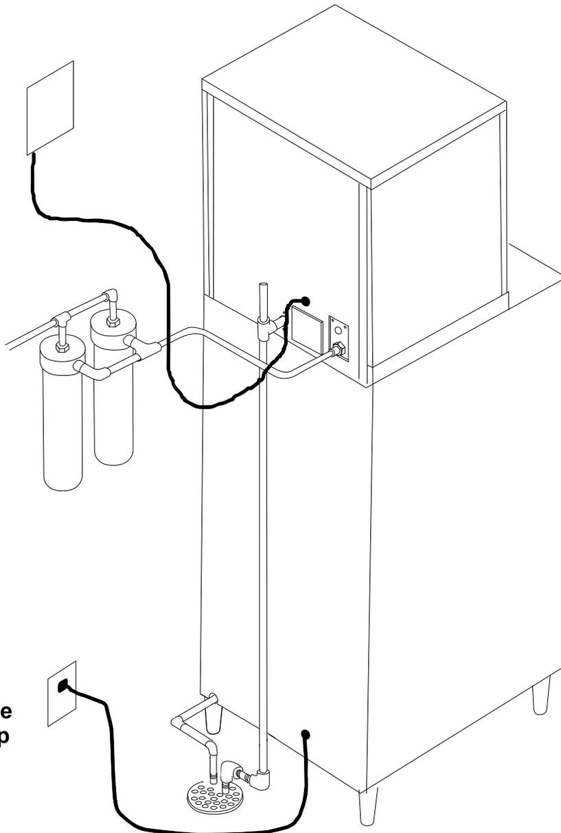
**Caution: Do not use a condensate pump in place of a floor drain.**
