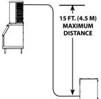
**15 ft. (4.5 m) Drop:** The maximum distance the Condenser or Condensing Unit can be below the ice machine.
