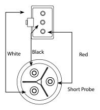
**Ohm water Level Probe and Wiring Harness**
