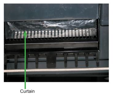
Front view of freezing compartment, arrow points to clear plastic curtain. After checking spray platform, pull curtain down to hang freely. This is its normal position.
