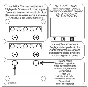
Master Switch. Move to ON (left side depressed) to make ice, OFF (centered) to shut off and WASH (right side depressed) for use in cleaning.
