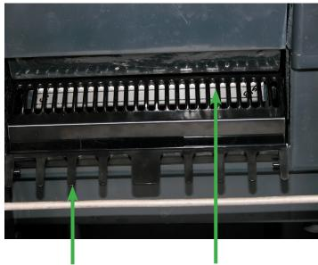
Front view of freezing compartment, right arrow points to Spray Platform, under the Cube Deflector. Push curtain back and check that it is in this position.
