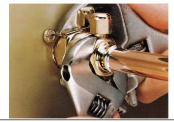
Note: As the couplings are tightened, the diaphragms in the quick connect couplings will begin to be pierced. As that happens, there will be some resistance to tightening the swivel nut.
