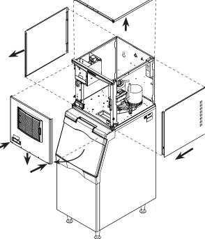
1. Locate and loosen the two screws at the bottom of the front panel.
