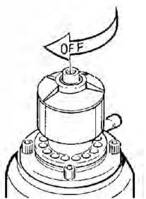
Inspect the top of the bearing. When new the grease is white, over time some gray will appear over the rollers, that is normal. Add grease to replace the gray grease or if gaps between rollers are visible. If grease is watery, all gray or rust is visible, have the bearing replaced. See the next page for more information.
