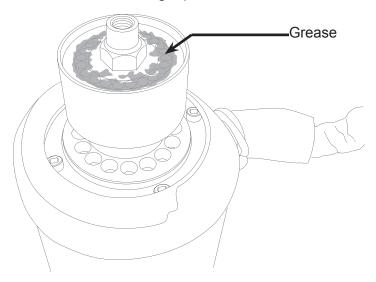
If the bearing only needs grease, or to confirm the quality of the grease low in the bearing, inject grease into the lower part of the bearing using Scotsman grease needle pn 02-3559-01 and Scotsman bearing grease cartridge, pn A36808-001. Be sure to inject grease evenly and thoroughly.
