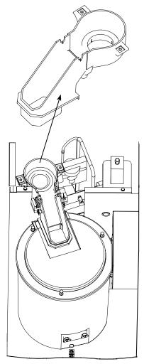
15. The ice chute can be cleaned in place. If complete removal is desired, use a Phillips screwdriver to remove the Hall Effect switch assembly from the ice chute.
