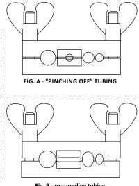
Fig. B - re-rounding tubing
