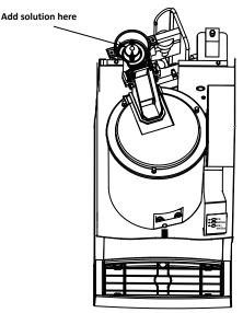
**Step 3** The ice machine will run a wash cycle, a series of rinse cycles and then stop. This entire cycle lasts approximately 30 minutes.
