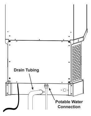
Connect drain tubing to the 3/4 inch FPT central drain fitting at the back of the cabinet. Use 3/4 inch rigid tubing, use material to meet local codes. The drain basin in the machine will act as an internal vent, no additional vent should be required unless there is a very long horizontal run. Drain tubing must pitch down 1/4 inch per foot to the building drain. Insulation of drain tubing is recommended for most environments.
