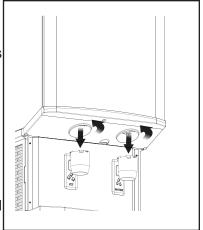
Twist ice and water chutes counterclockwise and pull down to remove.
