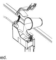
19. Mix a solution of 4 ounces of ice machine scale remover and 16 ounces of potable water. Use this scale remover solution to washout the water reservoir cover, ice discharge chute, ice chute cover, ice delivery chute, storage bin cover and inside of the ice storage bin. Slowly pour the cleaning solution down the bin drain.
