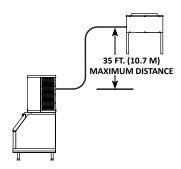
**35 ft. (10.7 m) Rise:** The maximum distance the Condenser or Condensing Unit can be above the ice machine.
