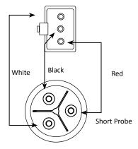
**Ohm water Level Probe and Wiring Harness**
